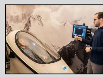
Once inside, the device delivers from 200 to 400+ patterned cycles of low pressure. A proprietary proportioning system assures that only filtered fresh air is allowed into the pod. A high performance regenerative vacuum blower suctions air out of the pod, while the proportioning system continuously vents fresh air back into it.
